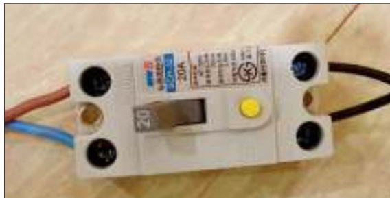
Use an ELCB (Earth leakage circuit breaker) for safety; long-time running can cause overheating
