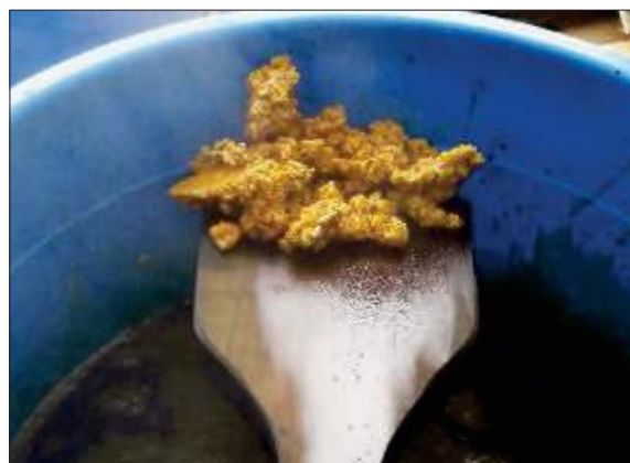
If initial water is too small, intense heat will solidify sulfur. Once solidified, it will not melt.
