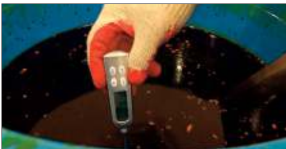
28. There are small particles of sulfur on the surface. Temperature started to drop. 15 minutes passed.
