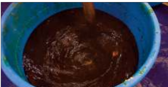
27. Mix while it is hot to melt sulfur.
