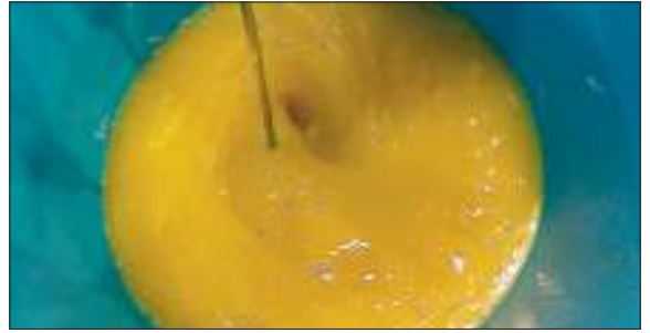
13. Color keeps changing and viscosity increases. 3 minutes passed.
