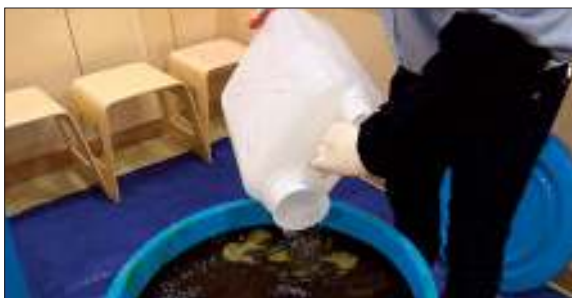
32. Add second water of 32 L (8.45 gal). Add 28 L (7.4 gal) if first water was 54 L (14.3 gal).
