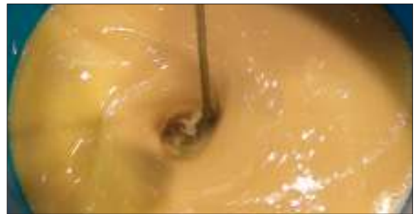
15. Color keeps changing and viscosity increases. 6 minutes passed.
