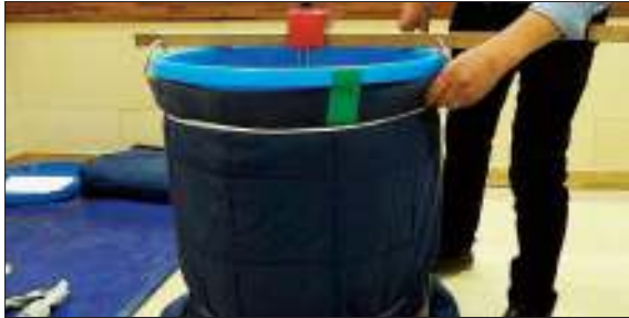
Wrap with insulation so that heat does not escape from the side or bottom.
