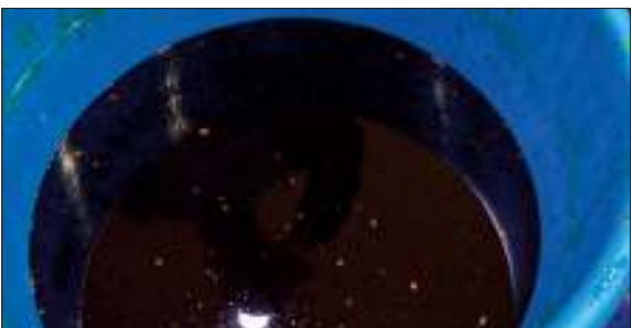
31. Sulfur has melted completely. Sulfur content is 40%. If you leave it as is, crystals will form when cold.
