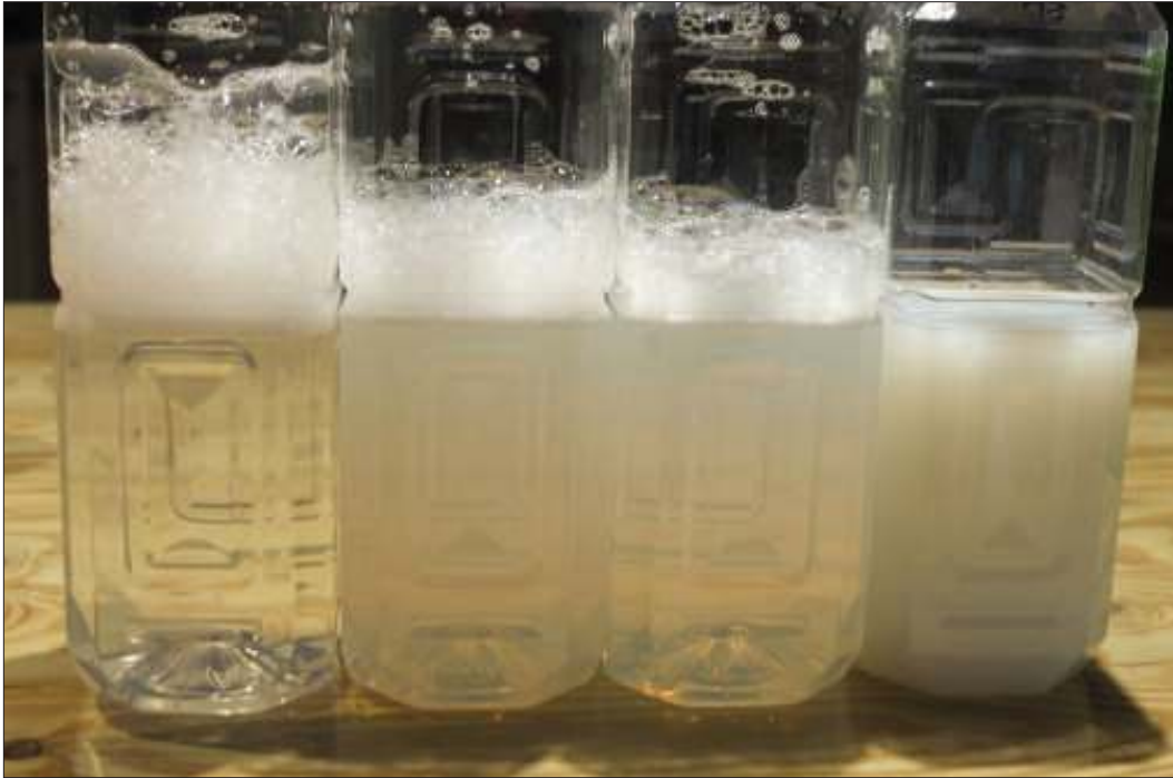
JADAM wetting agent water test. Mix a few drops of JWA, the water should remain clear. Shake, then there should be lots of foam
