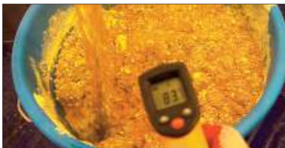
19. When temperature exceeds 80°C (176°F), sulfur starts to melt. 4 minutes passed.
