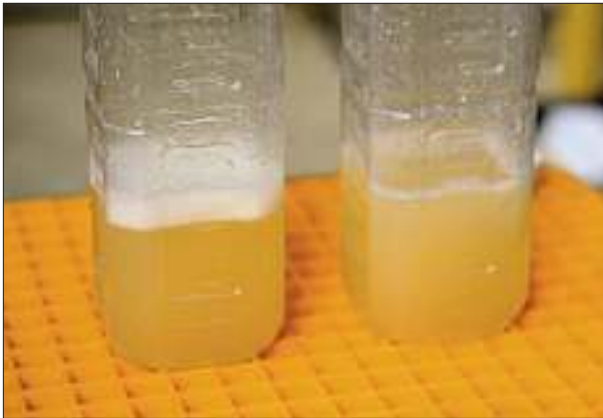
Chemical pesticides are also affected by water. Here, we tested a commercial mite pesticide with hard water. You can see there is little foam. This means weaker wetting power and thus less effectiveness as pesticide.
