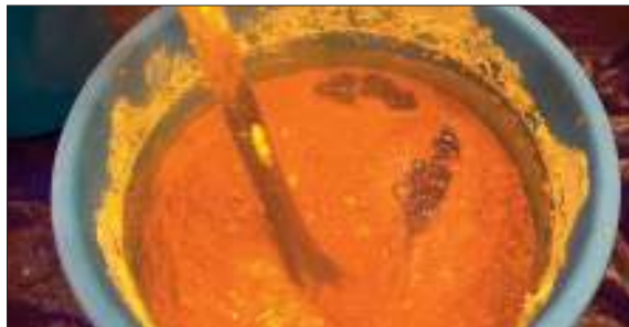
21. Liquefied sulfur becomes visible. 6 minutes passed.
