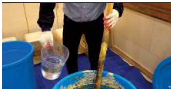
22. If water is too little or weather is too hot, it can over-boil. Have 2 L (0.53 gal) of water handy to pour in that case.
