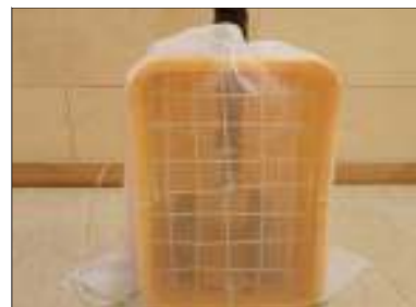
6. Tightly tie the opening of the bag. Put it in 5 t (1,320 gal) container and connect the motor.
